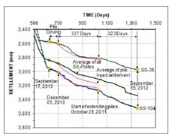
Fig. 6. Settlement of ground and piles at Substation
