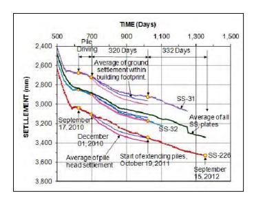
Fig. 5. Settlement of ground and piles at Maintenance Shop
