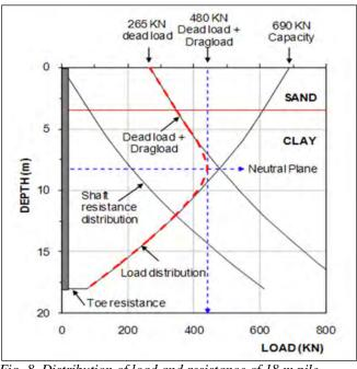
Fig. 8. Distribution of load and resistance of 18 m pile
