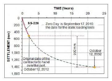
Fig. 7. Ground settlement vs. time at SS-226
